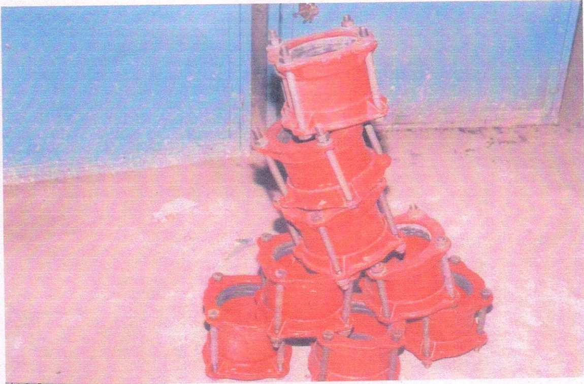
SOME FITTINGS - 6" JOHNSON JOINTS
