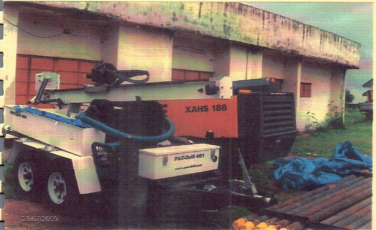
PAT 401 DRILLING RIG, COMPRESSOR AND SUPPORTING VEHICLES FOR RURAL WATER SUPPLY PROGRAM
