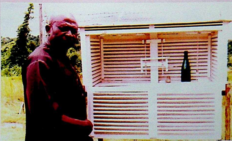
Stevenson Screen Housing the Thermometer, hydrometer and pitch evaporimeter for measuring temperature, humidity and evaporation at the meteorological station at Amawbia, Awka South L.G.A.
