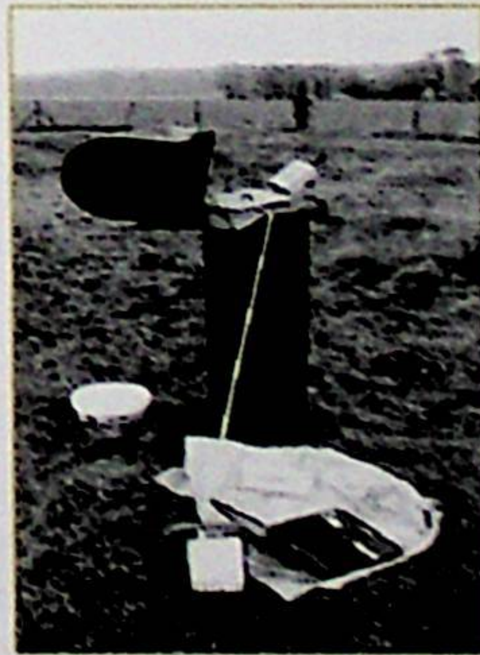
Sampling and water-level measurements in a standpipe
