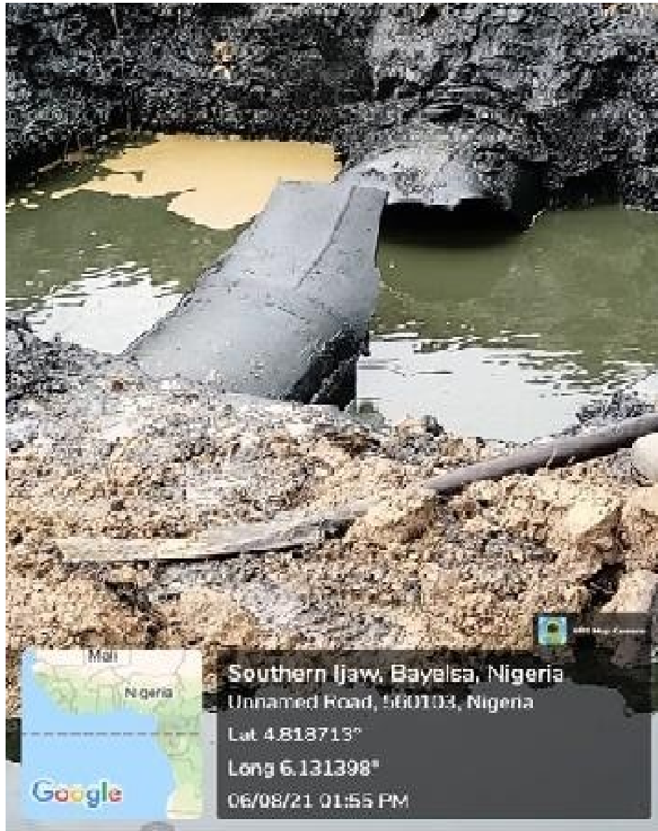
16" Nun River TL blown up using explosive. (sabotage)
