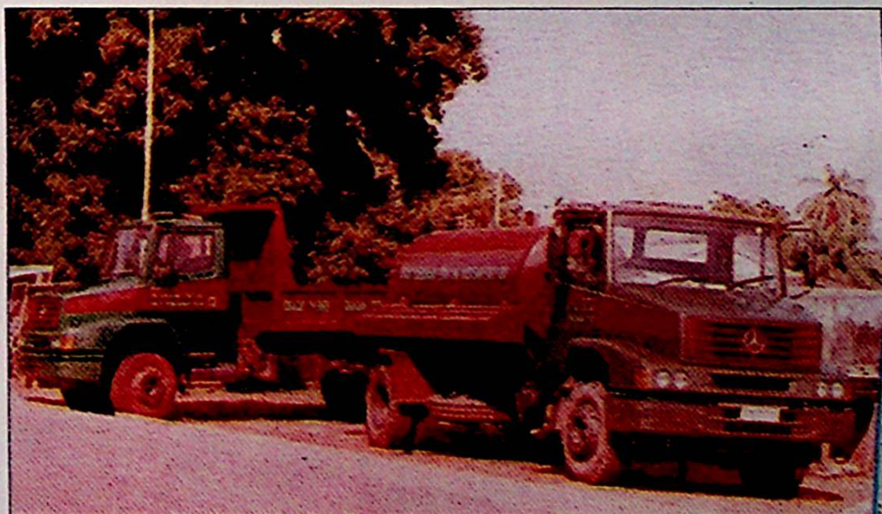
Septic Tank Emptier
